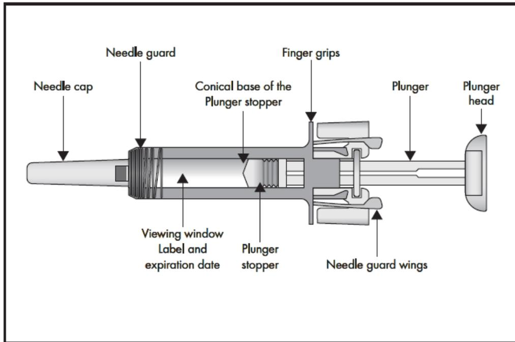
After the medication has been injected the needle guard will be activated to cover the needle. The needle guard is intended to protect healthcare professionals, caregivers, and patients from accidental needle sticks after the injection.
